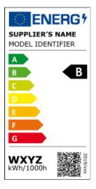
The design of the energy labels according to the new delegated regulation will be similar to the old version. What is new is that energy efficiency classes uniformly range from A to G for all products falling under the framework regulation 2017 /1369/EU and a QR code must be included on the label, which guides the consumer to the product entry of the light source in the product database if necessary.
