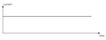
to 100%. Afterwards the battery remains being charged with the same current to ensure permanent 100% state of charge. The result of using this method is that the wasted energy from the constant charging heats up the battery.
