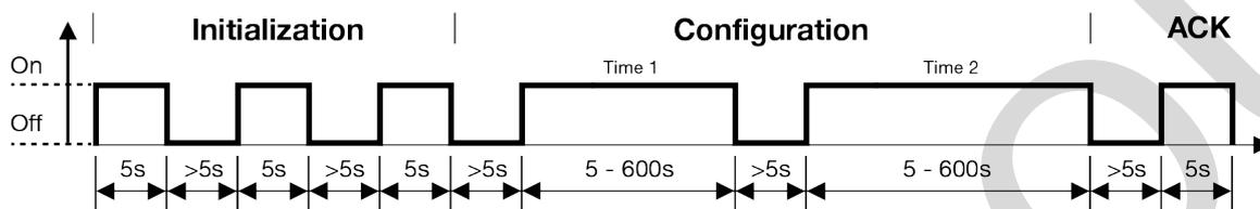
Programming mode 1 is used for setting the values Time 1 and Time 2 for Profile 1 of the chronoSTEP function. The values are defined by the length of the relevant On cycles in the Configuration block. 1 second for the On period equates to 1 minute for Time 1 or Time 2. The values are rounded to 5 minutes.
