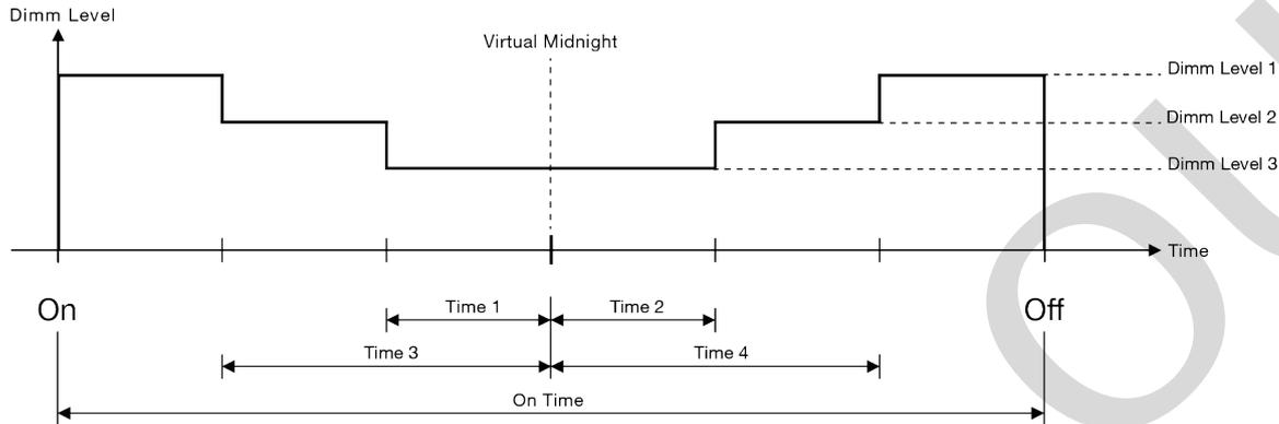
Profile 2 can be used to define four time intervals and three dimming levels. The combination of values allows more precise control of the dimming level at different times before and after Virtual Midnight.
