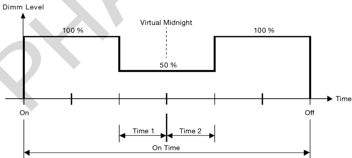
Two time intervals can be defined using Profile 1 (formerly U6M): Time 1 defines how many hours before Virtual Midnight the lighting is dimmed to a lower level; Time 2 defines how many hours after Virtual Midnight the dimming
