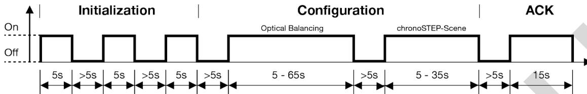
Programming mode 2 is used for selecting preset values for the Optical Balancing function and for selecting a scene from the chronoSTEP function. Which preset value or scene is selected is determined by the length of the relevant On cycle in the Configuration block. This is done by mapping the length of the On cycle onto a scale of 13 presets (for the Optical Balancing function) or a scale of 6 scenes (for the chronoSTEP function).
