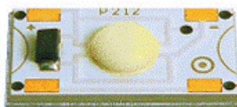
powerLED P211, damaged by dissolver waste gas
