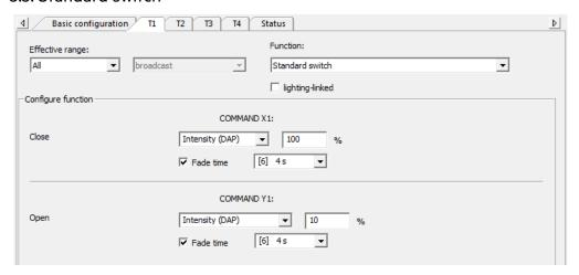
Depending on the state of the switch, the DALI XC will send its corresponding command X1 or Y1 onto the DALI line. The possible commands, which can be sent, are described further in the masterCONFIGURATOR manual.
