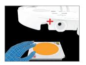
Inverse-polarity protection The polarity is clearly visible from the outside, even when the COB inserted
