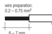
Inserting stranded wires / removing wires by lightly pressing on the push button.
