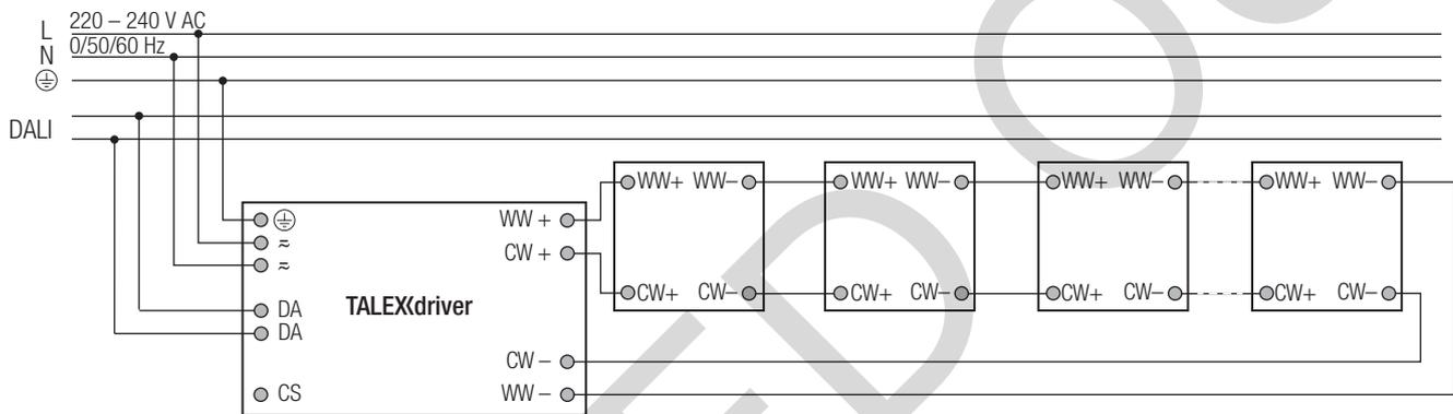
**Wiring type and cross section**
