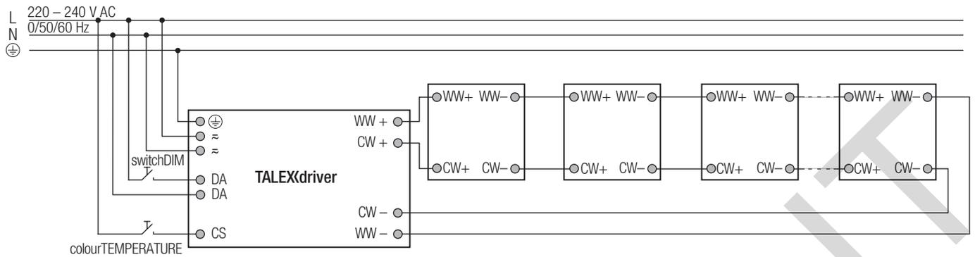
**Wiring diagram for DALI for the Engine QLE premium (with 4, 5 or 6 modules)**
