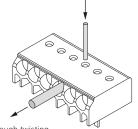
Loosen wire through twisting and pulling or using a  $\emptyset$  1mm release tool
