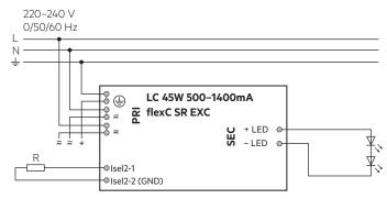
Device with loop through wiring function.
