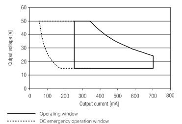
Make sure that the LED driver is operated within the given window under all operating conditions. Special attention needs to be paid at dimming and DC emergency operation as the forward voltage of the connected LED modules varies with the dimming level, due to the implemented amplitude dimming technology. Coming below the specified minimum output voltage of the LED driver may cause the device to shut-down.
