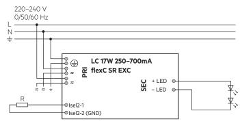
Device with loop through wiring function.
