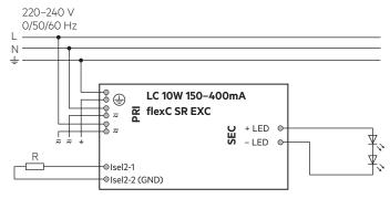
Device with loop through wiring function.
