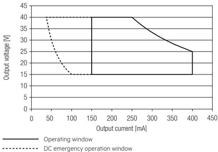
Make sure that the LED Driver is operated within the given window under all operating conditions. Special attention needs to be paid at dimming and DC emergency operation as the forward voltage of the connected LED modules varies with the dimming level, due to the implemented amplitude dimming technology. Coming below the specified minimum output voltage of the LED Driver may cause the device to shut-down. See chapter "6.7 DC emergency operation" for more information.
