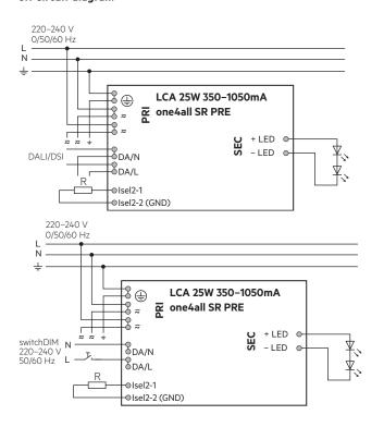
Device with loop through wiring function.
