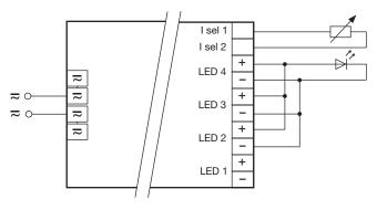
Parallel circuit of 4 channels (max. output current 1,600 mA)
