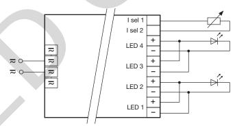
Parallel circuit of 3 channels (max. output current 1,200 mA)
