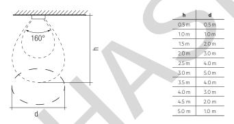
Diameter of the detection cone as a function of height at maximum detection area without taking objects in the room into consideration. Stationary objects (walls, tables, floor-standing luminaires, etc.) located in the direct view of the sensor change the characteristics of the detection area.
