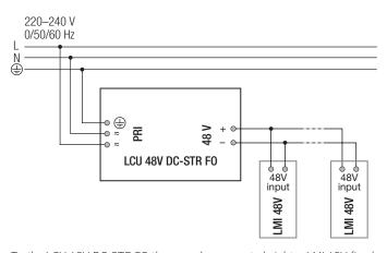
To the LCU 48V DC-STR FO there can be connected eighter LMI 48V fixed output version or LMI 48V dimmable version.
