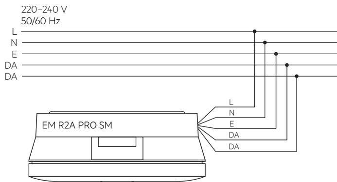
Note: Battery must be connected before mains connection.
