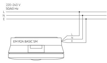
Note: Battery must be connected before mains connection.
