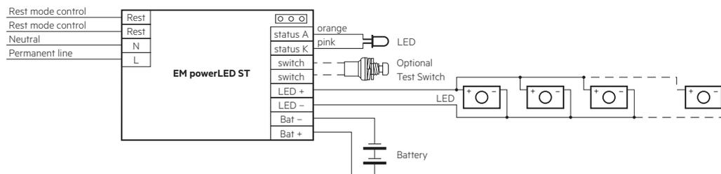
Take care that the LED is connected with the right polarity. LED that are connected to the EM powerLED PRO EZ-3 devices should have a reverse polarity protection device such as a schottky diodes fitted, otherwise irreversible damage could occur if the LED is connected in reverse polarity. Any protection device must be capable of handling in excess of 1,000 mA.
