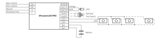
Take care that the LED is connected with the right polarity. LED that are connected to the EM powerLED PRO EZ-3 devices should have a reverse polarity protection device such as a schottky diodes fitted, otherwise irreversible damage could occur if the LED is connected in reverse polarity. Any protection device must be capaple of handling in excess of 1,000 mA.
