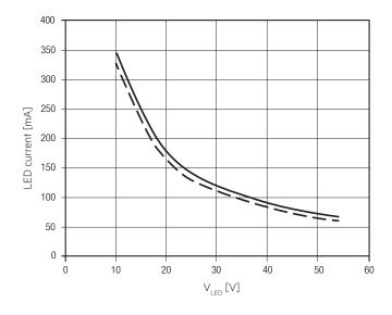
LED current at nominal battery voltage and min. battery discharge current
