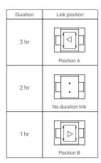
Emergency lighting LED driver supplied with duration link in 3 hours position (position A).
