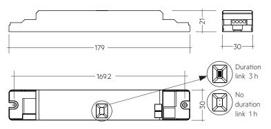
Note: LED driver supplied with duration link in 3 hours position. Remove duration link for 1 hour duration. Duration link must be set before battery and mains connection.
