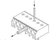
Loosen wire through twisting and pulling or using a Ø 1mm release tool
