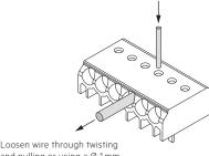
and pulling or using a Ø 1mm release tool
