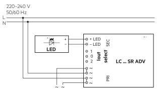
Device with loop through wiring function.
