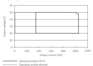
Make sure that the LED driver is operated within the given window under all operating conditions. Special attention needs to be paid at dimming and DC emergency operation as the forward voltage of the connected LED modules varies with the dimming level, due to the implemented amplitude dimming technology. Coming below the specified minimum output voltage of the LED driver may cause the device to shut-down. See chapter "6.9 DC operation" for more information.
