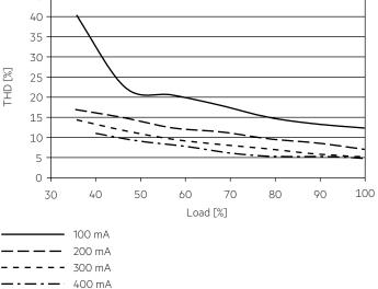
100 % load corresponds to the max. output power (full load) according to the table on page 2. Values measured at 230 V, 50 Hz.
