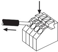
Press down the "push button" and remove the cable from front.
