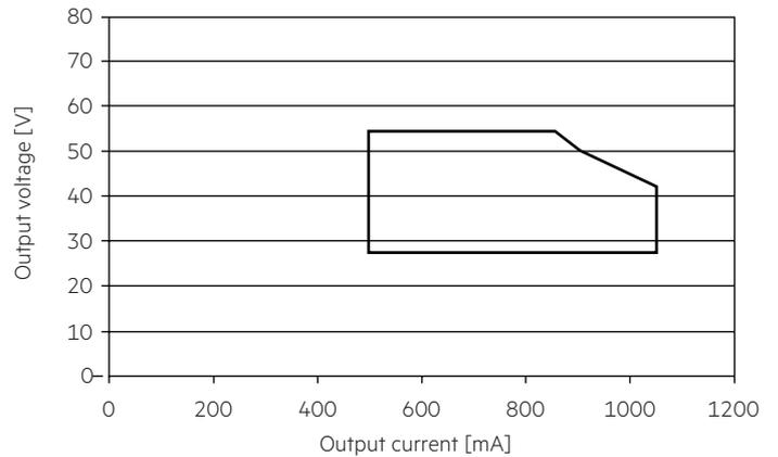
Make sure that the LED driver is operated within the given window under all operating conditions.
