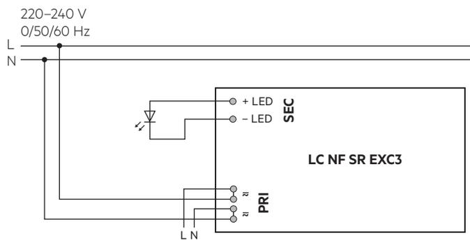
Device with loop through wiring function.
