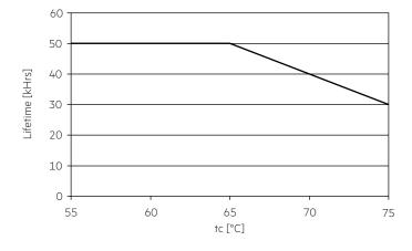
$The \ LED \ driver \ is \ designed \ for \ a \ lifetime \ stated \ above \ under \ reference \ conditions \ and \ with \ a \ failure \ probability \ of \ less \ than \ 10 \ \%.$
