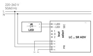
Device with loop through wiring function.
