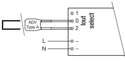
**650 mA:** Terminal 0 and 2 connected with resistor ADV Plug Type D BR (article number: 28001774)
