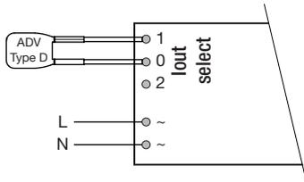
**600 mA:** Terminal 0 and 2 connected with 0 Ω wire (max. 6 cm length) or resistor ADV Plug Type A BR (article number: 28001771)
