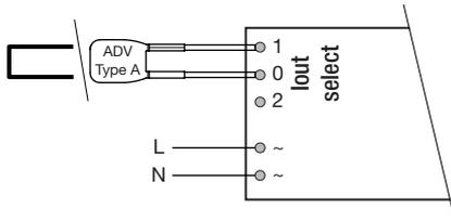
**550 mA:** Terminal 0 and 1 connected with resistor ADV Plug Type D BR (article number: 28001774)
