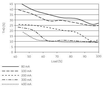
100 % load corresponds to the max. output power (full load) according to the table on page 2. Values measured at 230 V, 50~Hz.
