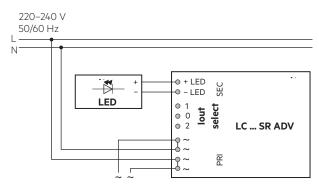
Device with loop through wiring function.
