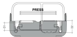
Depending on the used flaps of the terminal following cable jacket diameter difference between the side D2 and D1 terminals is recommended:
