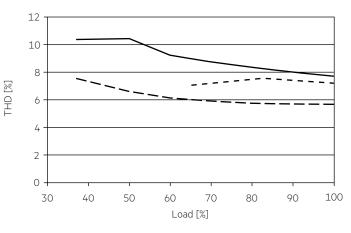
100 % load corresponds to the max. output power (full load) according to the table on page 3.
