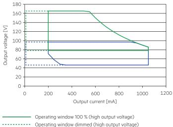
Operating window dimmed (low output voltage) Make sure that the LED driver is operated within the given window under all operating conditions. Special attention needs to be paid at dimming and DC emergency operation as the forward voltage of the connected LED modules
