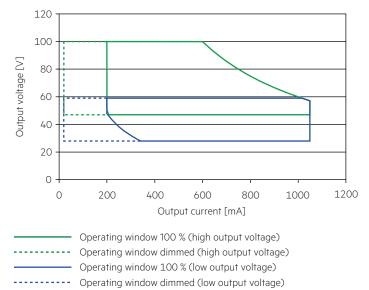
Make sure that the LED driver is operated within the given window under all operating conditions. Special attention needs to be paid at dimming and DC emergency operation as the forward voltage of the connected LED modules varies with the dimming level, due to the implemented amplitude dimming technology. Coming below the specified minimum output voltage of the LED driver may cause the device to shut-down.
