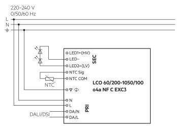
switchDIM with high voltage output (HV)
