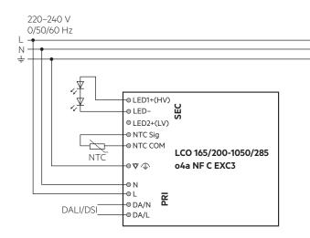
220-240 V 0/50/60 Hz L Ν ÷ ``{{ © LED1+(HV) SEC • LED-● LED2+(LV) - NTC Sig -• NTC COM LCO 165/200-1050/285 NTC o4a NF C EXC3 • 🌣 🛆 ΘN • L PRI ● DA/N DALI/DSI ● DA/L
