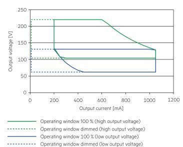
Make sure that the LED driver is operated within the given window under all operating conditions. Special attention needs to be paid at dimming and DC emergency operation as the forward voltage of the connected LED modules varies with the dimming level, due to the implemented amplitude dimming technology. Coming below the specified minimum output voltage of the LED driver may cause the device to shut-down.
