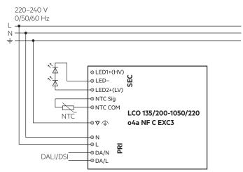
switchDIM with high voltage output (HV)
