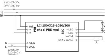
For wiring in dimming operation with ready2mains refer to the ready2mains Gateway datasheet.
