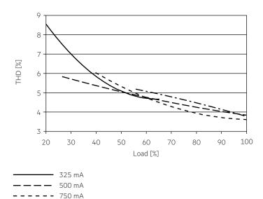
100 % load corresponds to the max. output power (full load) according to the table on page 2.
