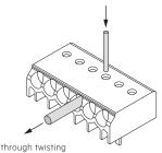
Loosen wire through twisting and pulling or using a Ø 1mm
