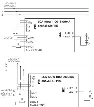
Device with loop through wiring function.
