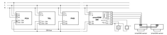
Several smartDIM sensors can be connected in parallel.
