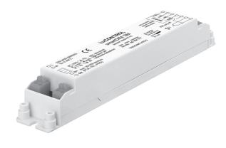
Digital DSI control module for controlling up to 25 digital, electronic DSI devices. The smartDIM SM allows user friendly dimming and ON/OFF switching via standard single- or double-gang momentary switches. Any number of switches can be connected in parallel to the smartDIM SM thus enabling operation from several points. By connecting a smartDIM sensor, the connected PCA/TEL/PHD devices can be switched automatically and the ambient lighting can be regulated via the control line.
