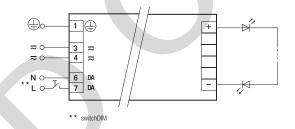
LED's have to be connected as shown above to work properly. It is possible to connect a different number of LED's on two circuits (like on top picture). The minimum power load has to be connected. Otherwise the LED control gear will switch off.
