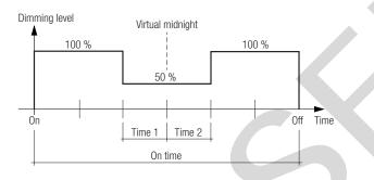
Time 1 and Time 2 can be set via ON/OFF cycles of the mains supply voltage (programming mode 1).
