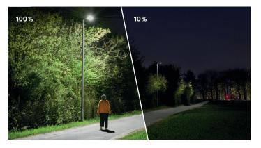
Many paths and squares are used only sporadically during twilight and after dark, yet lighting is a key safety factor. Light is proven to reduce the number of criminal attacks. The solution is to dim luminaires to, for example, 10% when the paths are not in use. This reduces energy consumption and pollution without jeopardising the safety of residents through a complete shutdown of the luminaires.
