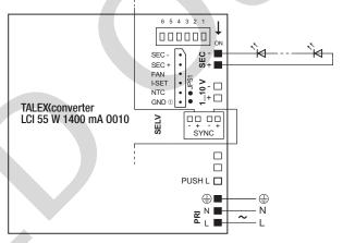
① common ground (GND) for FAN, I-SET and NTC
